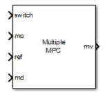
As for the MPC Controller block, at each control instant the Multiple MPC Controllers block receives the current measured plant output, reference, and measured plant disturbance (if any). In addition, it receives a switching signal that selects the *active controller* from among a list of two or more candidates. The active controller then solves a quadratic program to determine the optimal plant manipulated variables for the current input signals.
