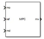
The MPC Controller block receives the current measured output signal (mo), reference signal (ref), and optional measured disturbance signal (md). The block computes the optimal manipulated variables (mv) by solving a quadratic program (QP).
