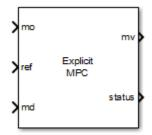
Like the MPC Controller block, the Explicit MPC Controller block uses the following input signals:
